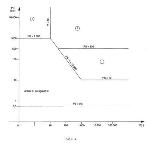
Figure 2.3: Conformity Assessment Table 4 for Vessels (Liquid, Group 2)
