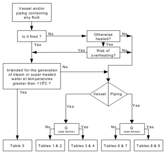
Q. Does the vessel or piping contain liquid whose vapour pressure at the maximum allowable temperature is not more than 0,5 bar above normal atmospheric pressure?
