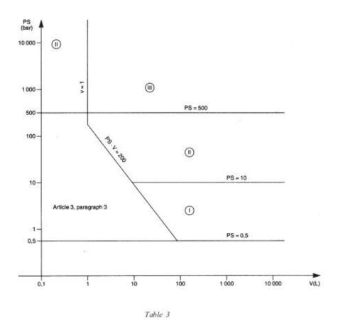
Figure 2.2: Conformity Assessment Table 3 for Vessels (Liquid, Group 1)
