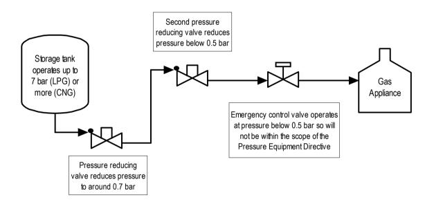
Figure 4.1: Example of an End-User Installation
