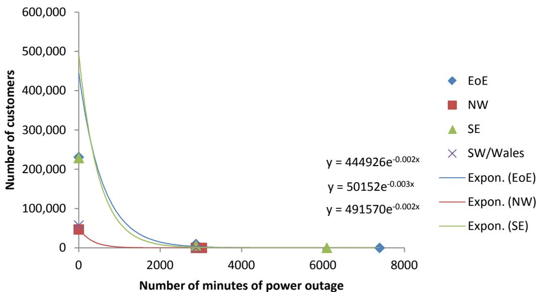
**Figure 12.2 Graph showing trend lines and formulas used to calculate median number of hours affected (minutes ÷ 60)**
